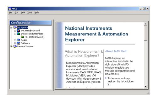
You can also test the different outputs channels with this program by running the Test Panel application. Right click the PCI-6503 in the Devices and Interfaces tree and select Test Panel.
