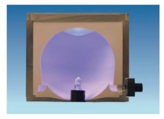
device for measuring optical radiation. The interior surface of the integrating sphere is perfectly diffusing and has spatially uniform reflectance. The radiant exchange from diffuse surface to diffuse surface integrates the light, resulting in equal radiance at any point on the sphere wall.
