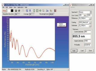
The AvaSoft-Thinfilm supports multiple channels and 8 time series for layer thickness and fit quality.
