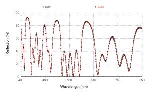
The software measures film thickness and optical constants (N & K) up to 5 layers.
