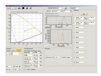
Radiated optical energy, as measured by Avantes spectrometers, can be quantified as a radiant flux, a measure in energy per second (Watt) radiated from a source. The radiated optical energy can be correlated with human vision (photometry) as defined in the CIE to obtain a spectral luminous efficiency function to characterize the vision of an average human observer.
