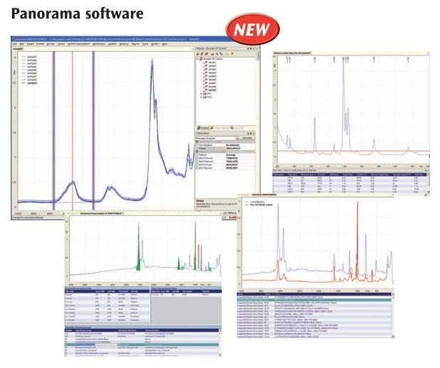
Panorama software works with all AvaSpec-USB2 spectrometers. All 2D and 3D spectroscopic data can be manipulated with just a few mouse clicks. Manipulation operations can easily be undone and redone unlimited times. Frequently used mathematical operations are automatically stored in a math operation history and can be applied to subsequent data sets.
